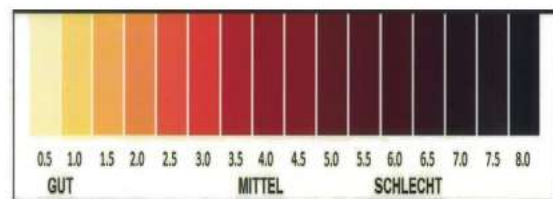
Colour Scale ASTM D 1500
